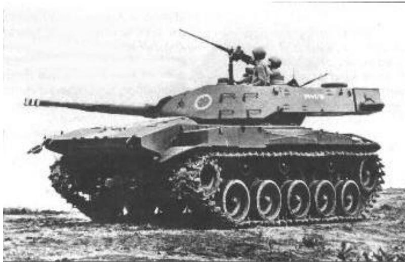
**One of the two M-41B with Cockerill/Engesa of 90mm cannon in tests. Notice the chassis lengthening in the rear part for the new motor diesel, and the same original model tower M-41 with new cannon. Credit for photo: Bernardini S/A**
