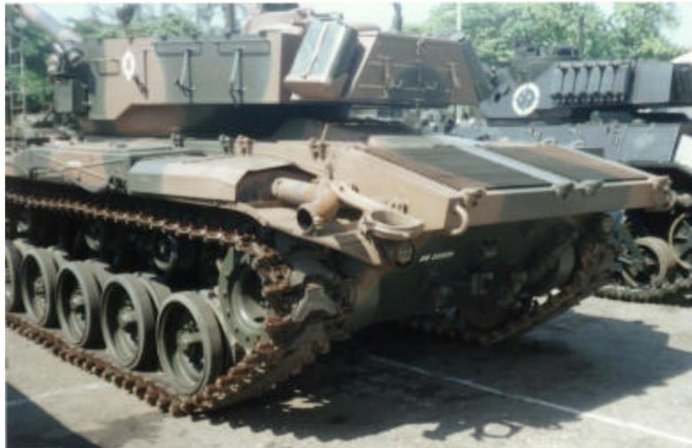
**Detail of the rear of M-41 C. The motor compartment increased and only one leakage instead of the two in the original model. Credit for photos: Author's collection**
